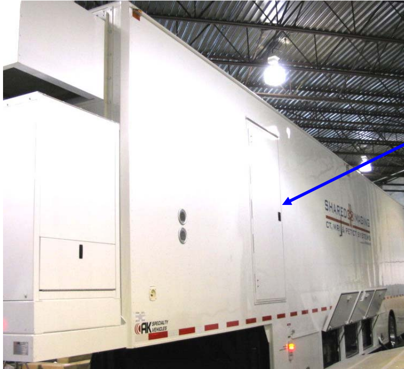
Figure 22: Emergency Exit / Service Door
