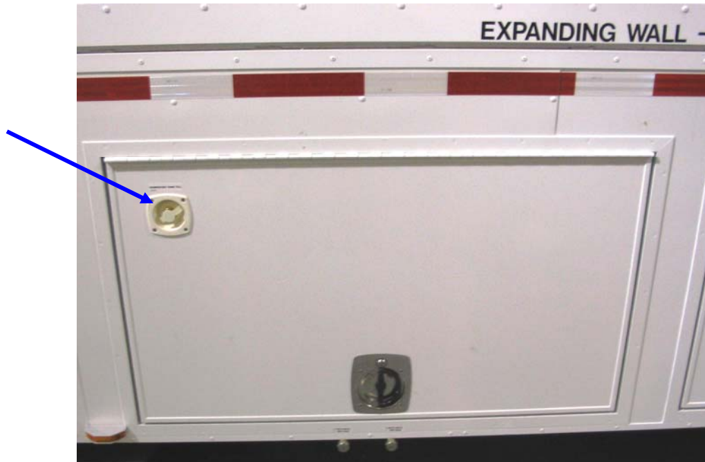
Figure 19: Fresh Water Tank Fill
