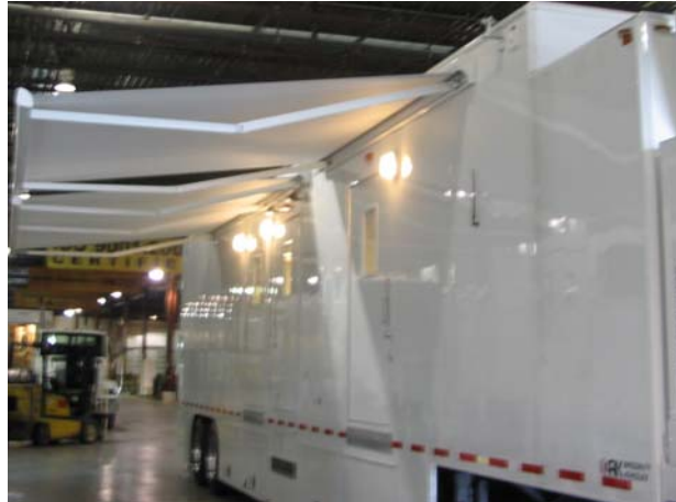
Figure 33: Entry Door Lighting
