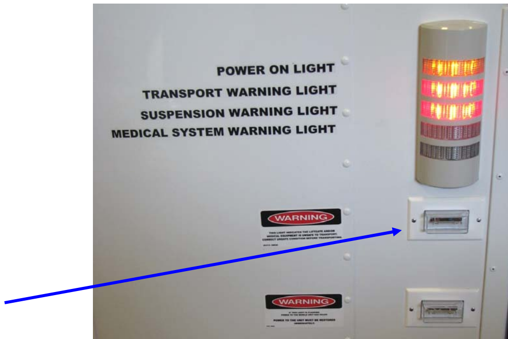
Figure 56: Lift Transport Warning Strobe
