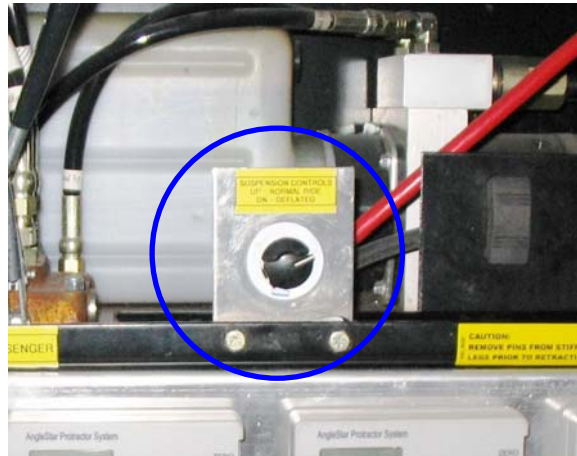
Figure 47: Air Bag Controls
